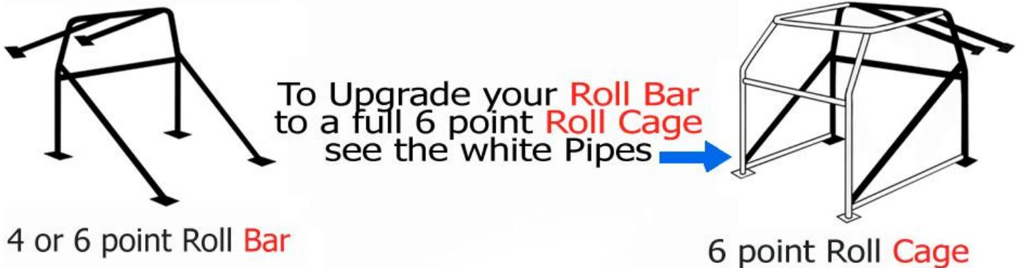
A 4-point cage is what is typically referred to as the "roll bar". It's a single tube starting from the vehicles floor, wraps up the car's B-pillar, across the roof, and back down the opposing B-pillar. Generally two tubes (one on each side) will come down from high on the B-pillar tube down to the floor; close to the drivers foot-well. (See figure below)
